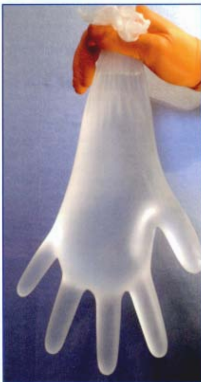
Vinyl gloves undergoing a water test
